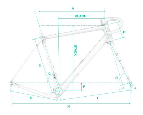
The KAHA features a Gravel Racing geometry designed for balance and stability at speed across any terrain. The double dropped chainstays delivers tire clearance up to 50mm Front & 47mm Rear (700C/650B).
